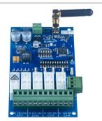
PCR43305R 5-Channel Receiver with Relay Outputs
