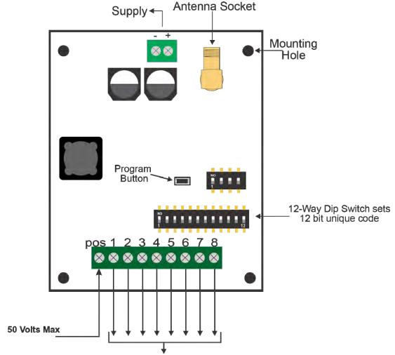
Voltage into the POS terminal will appear on these terminals when the channel is activated. Max switching current is 120 mA For higher switching current please see the datasheet for A2982LW
