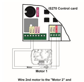
the motor 2 encoder wire to "Motor 2 Encoder" terminal
