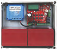
Control card, Solar panel, Battery & Regulator with MPPT
