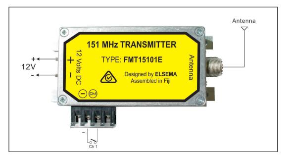
Inputs of the transmitter should be voltage free contact closure only.
