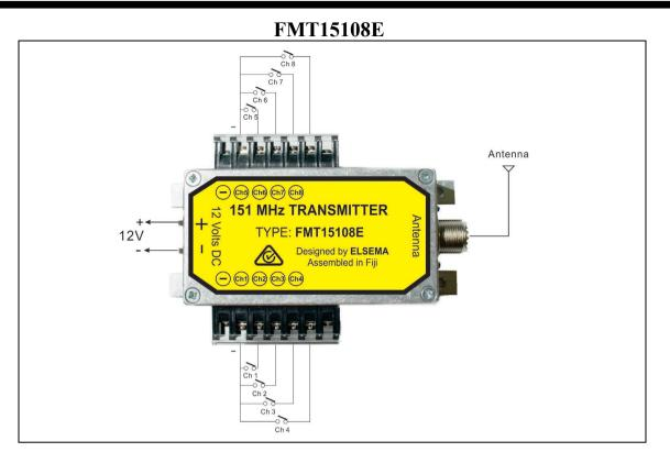
Inputs of the transmitter should be voltage free contact closure only.
