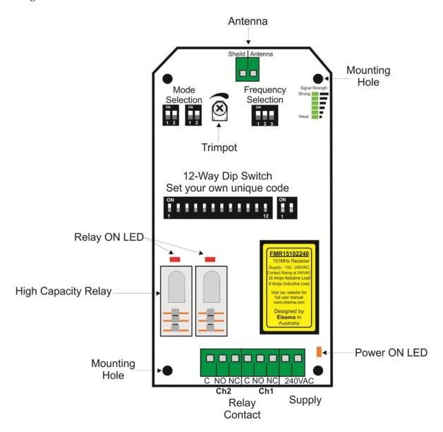
Relay output is voltage free contact
