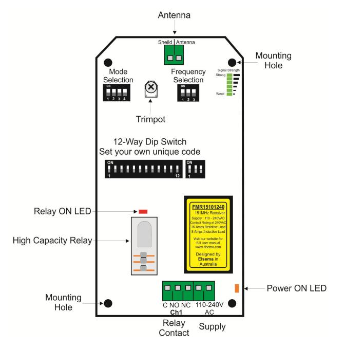
Relay output is voltage free contact
