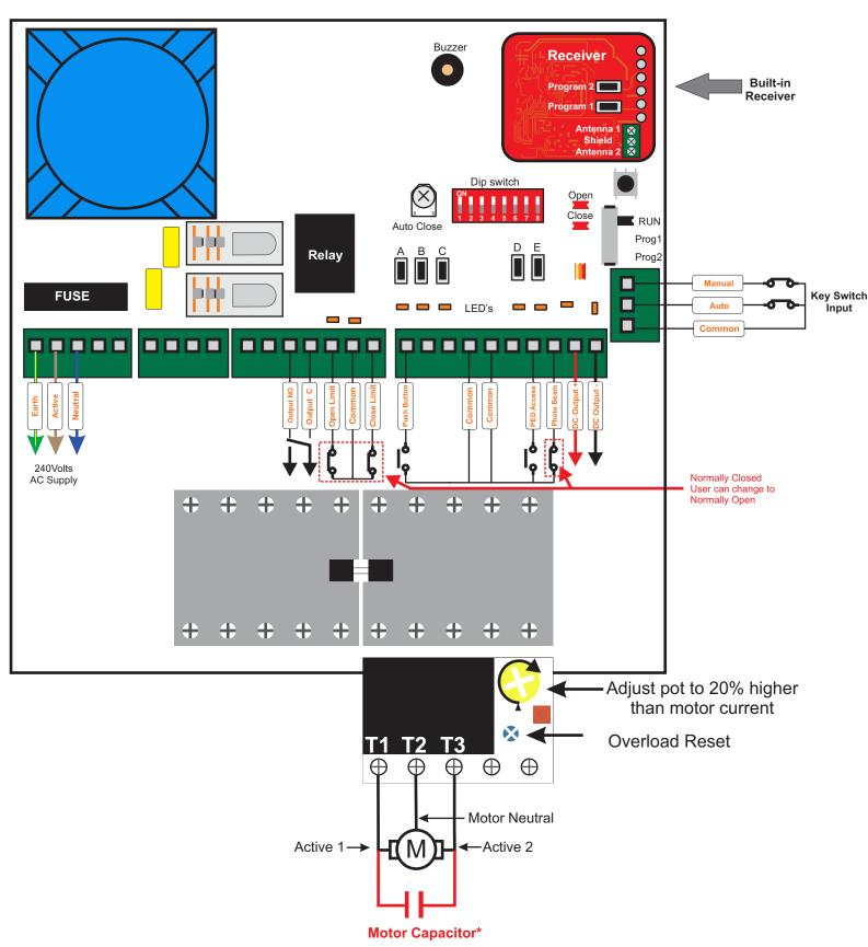
Check motor specifications before connecting. Some motors have internal capacitors
