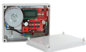
Intelligent control box with built-in receiver.
